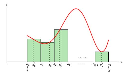
Each of the rectangles has height of  $f(x_i^*)$  and we could then use the area of each of these rectangles to approximate the area as follows.
